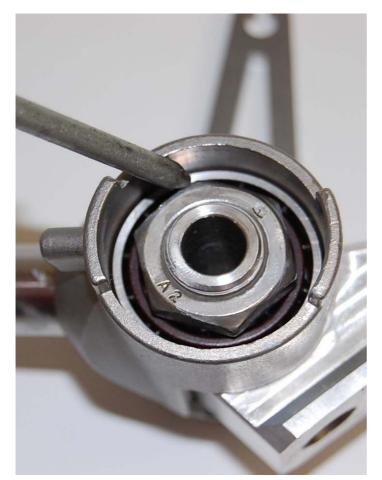
To prevent unnecessary wear, you should check at least once a year that the bearing is still sufficiently greased, and if necessary apply more grease.
