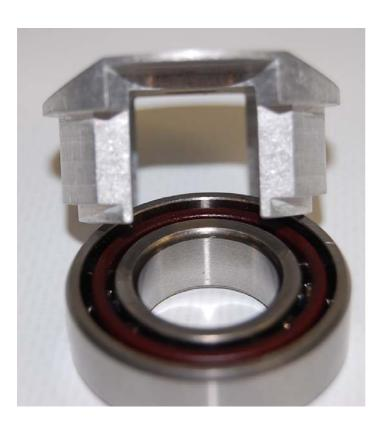
Angular contact ball bearings are designed to withstand large forces in one axial (vertical) direction. Normal ball bearings cannot do this. Because these forces can only be resisted in one direction, it is of great importance that the bearing is mounted correctly.
