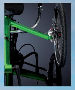
Wings at the front of Challenge Trikes are more than a stunning visual. First, the forward angled design allows stepping up close to the seat, then sitting down easily rather than falling in.
