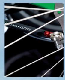
Aero profile tie rods feature clean internal cable routing, and the double thread arrangement gives easy toe-in adjustment at the ends. Elegantly finished in anodized black.
