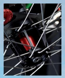
Challenge Trike hubs are loaded with innovation. A stylish and strong tapered shape with cut-outs to save weight and also give a look "inside." 32 traditional style spokes for easy service and oversize inside bearings give better heat transfer and long life under high side load cornering forces.
