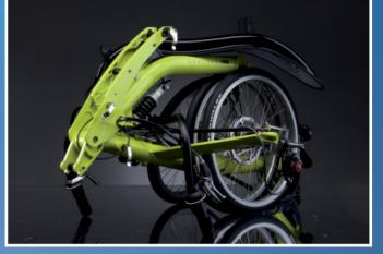
The Challenge Alizé is a folding trike. Fits behind the seats of a Smart car without removing the boom. Disassambled, the trike takes even less space.
