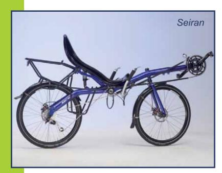
Seiran's big wheels roll fast and easy on smooth roads and in the rough. Weight distribution is perfect for optimum traction, and steering dynamics that are just right. Challenge's curved frame design keep the seat height reasonable, and temper the crank elevation for easy acceptance. Seirans can be built for extreme touring in the rough of the world, or with light SL type components for the fast club ride with the added bonus of rear suspension smoothness.
